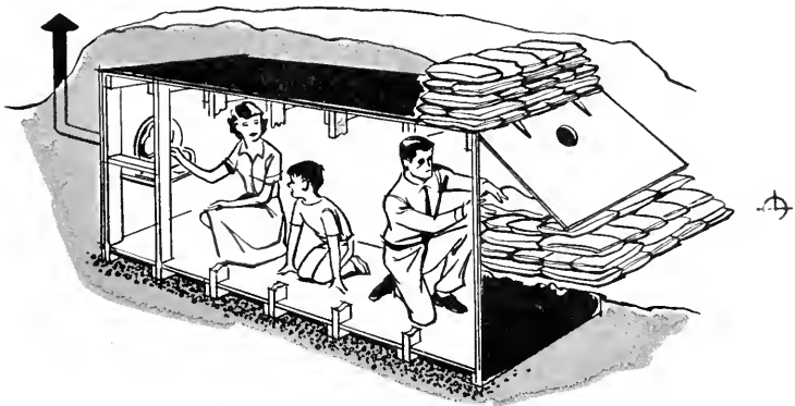
This backyard plywood shelter can be built partially above ground and mounded over with earth, or be built totally below ground level. A gravel drain under the shelter and a ditch outside help keep it dry. The family blocks the entrance with sandbags after entering the shelter.
